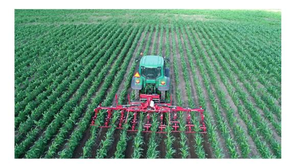
The CMN Steering Frame is designed to mount between the tractor and the implement.
