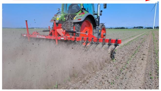
**CMN Star-cleaner** – The optimal solution for breaking up the earth's crust and for mechanical weed control. The CMN Star-cleaner with three-point suspension is available in 3, 6, 8, 9, 10 and 12m working widths.
