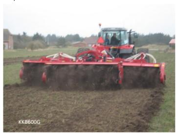
This means that the machine can adapt to unevennes in the field. The effective working width of the side rotor is 1.6m and that of the middle rotor is 3m. This means that the machine will overlap by 10cm.
