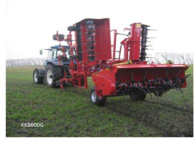
After the cultivator follows the patented PTO driven rotor system.
