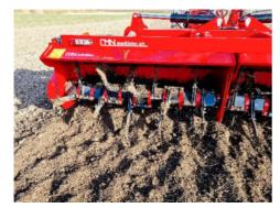
All machines are equipped with automatic coupling. In fields with many stones or very clayey soil it is advisable to provide the rotor with an additional rubber suspension on the tines. This counteracts breaking the security bolts and the machine gets a smoother running, at the same time.
