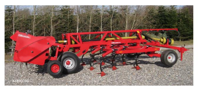
The KKB**\$**400SG model is foldable. It has a lot in common with its predecessor, the KKB400SG, but also has additional advantages. In addition to the reduced transport width, the rotor of the couch grass killer is fitted with a parallelogram suspension. This means the depth of the rotor can be varied additionally in relation to the tines. The rotor is divided in 2 sections, each one is centered. This allows the rotor to adapt to unevenness in the field.
